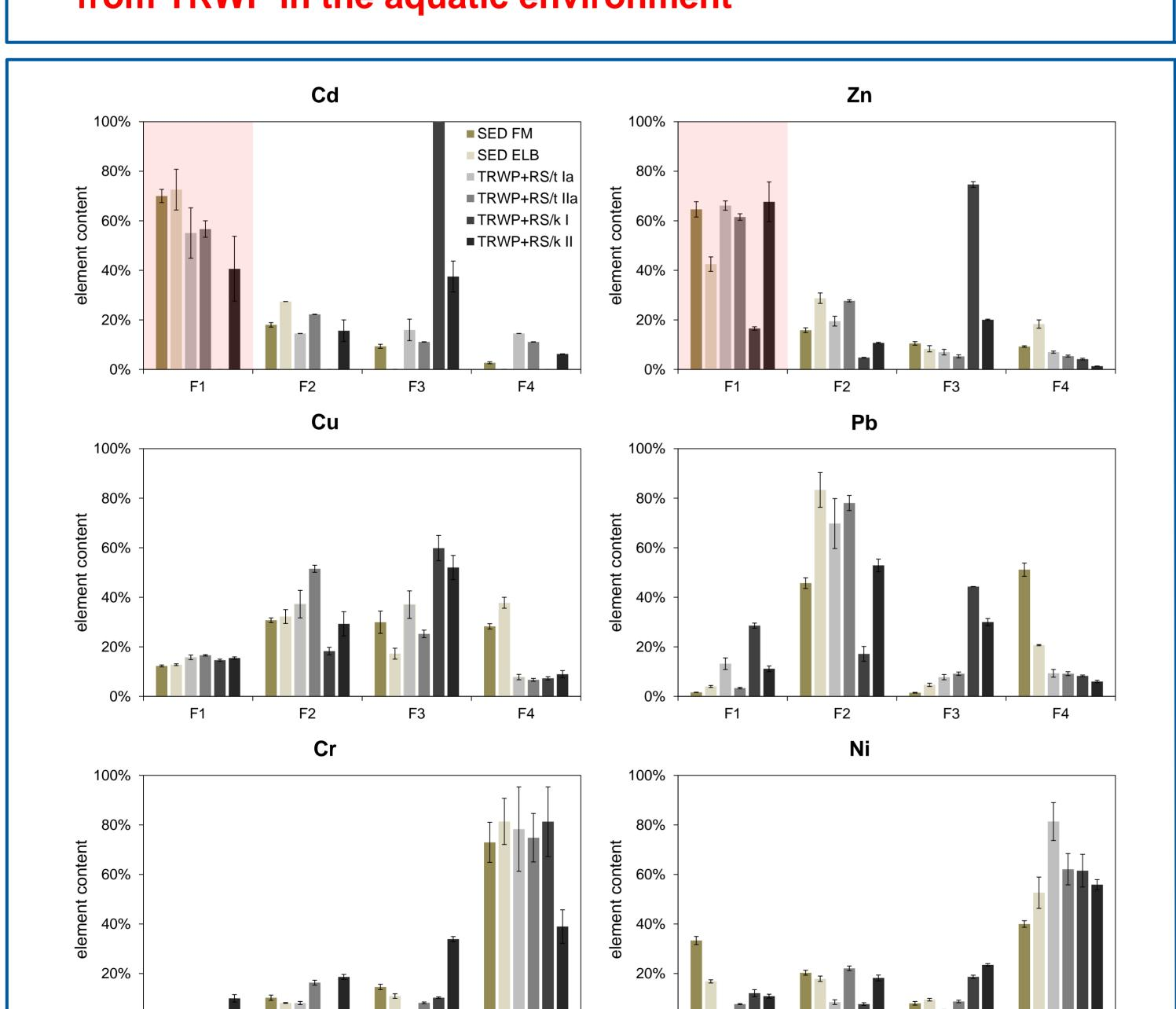
Fig. 1: Relative element distribution of Cr, Ni, Cu, Zn, Cd and Pb as derived from BCR extraction for sediment samples of the Freiberger Mulde (SED FM) and Elbe (SED ELB), as well as for TRWP+RS/t from the Elbtunnel (Ia = beginning, IIa = middle) and TRWP+RS/k from kart tracks (I & II). Standard deviation given as uncertainty.
