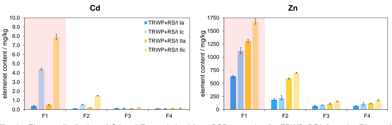
Fig. 2: Element distribution of Cd and Zn as derived from BCR extraction for TRWP+RS/t from the Elbtunnel (I = beginning, II = middle) before (a) and after (c) incubation experiments. The uncertainty is given by the first standard deviation. Standard deviation given as uncertainty.
